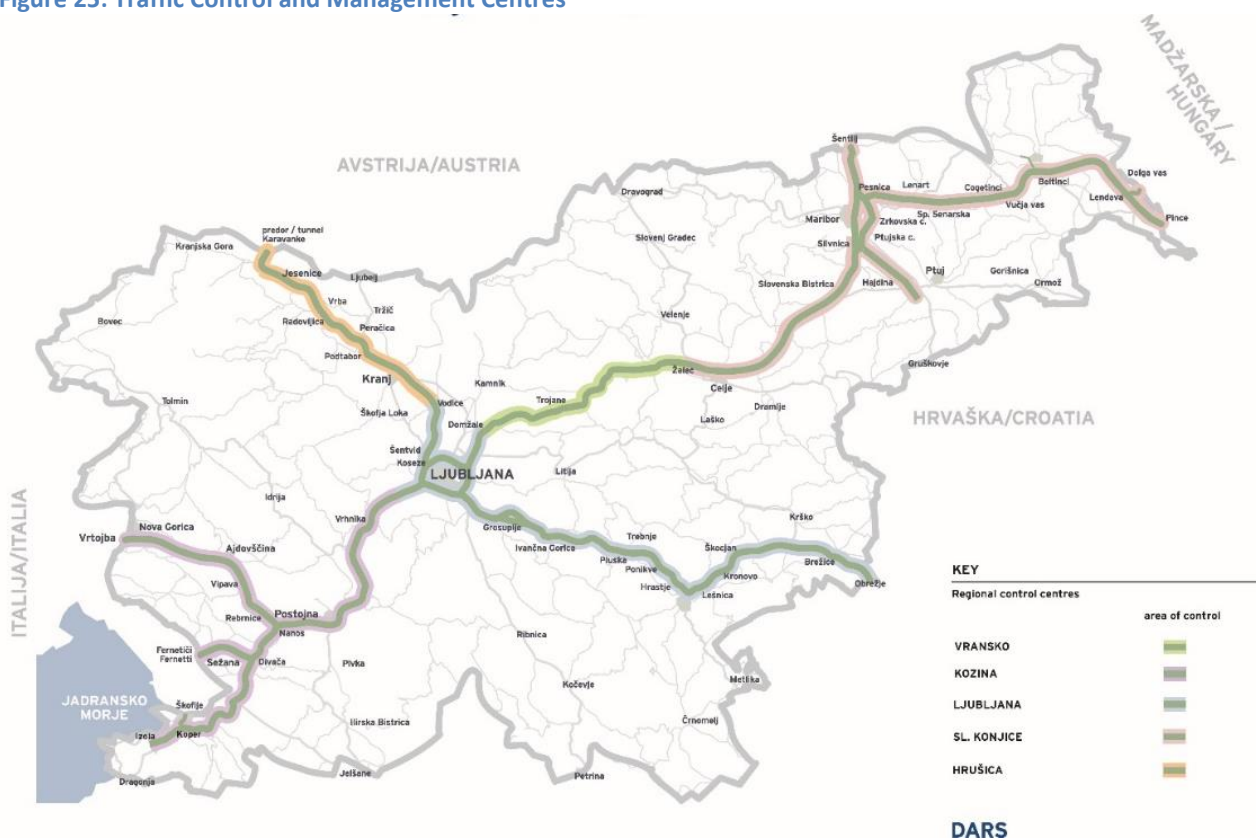
Figure 25: Traffic Control and Management Centres
